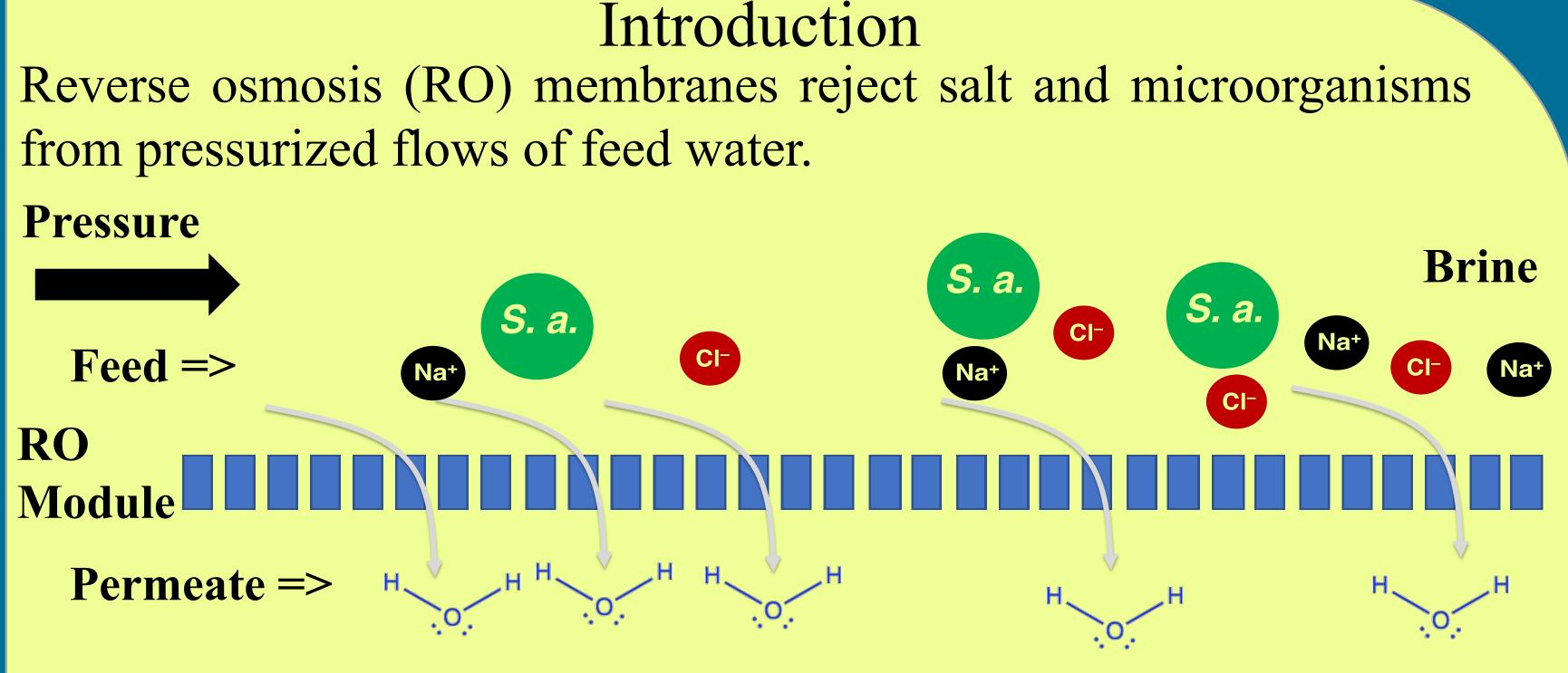
The rejected salt and microorganisms concentrate downstream in the RO module into the brine solution.
